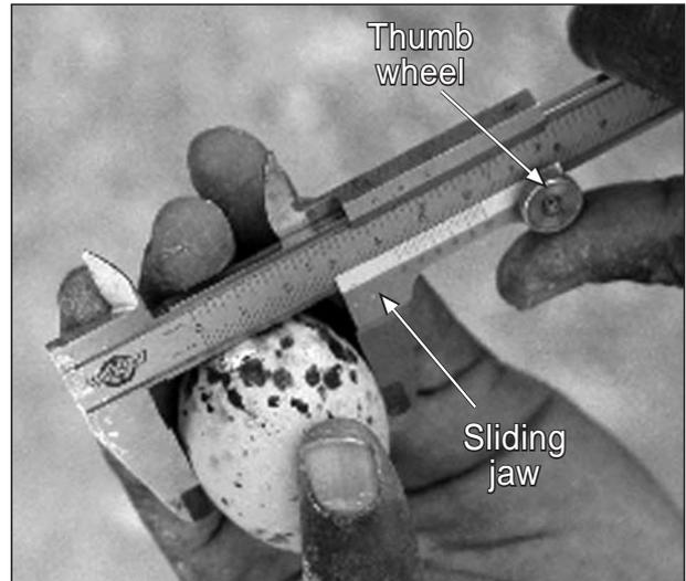
Figure A.3.2. Detail of the graduation system of the vernier calipers
