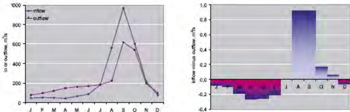
**Figure 2.** LEFT: The monthly inflow and outflow of the Sélingué reservoir ( $m^3/s$ ), averaged over the period 1982-2003; source: EDM. RIGHT: Using the same data, the difference as  $m^3/s$  between monthly inflow and outflow in the Sélingué reservoir. From Zwarts, I., Cissé, N. & Diallo, M (2007) *Hydrology of the Upper Niger- In: Zwarts, L., Beukering van, P., Kone, B. and Wymenga, E. (eds.), The Niger, a lifeline. RIZA/Wetlands International/IVM/A&W, pp. 15-42.*
