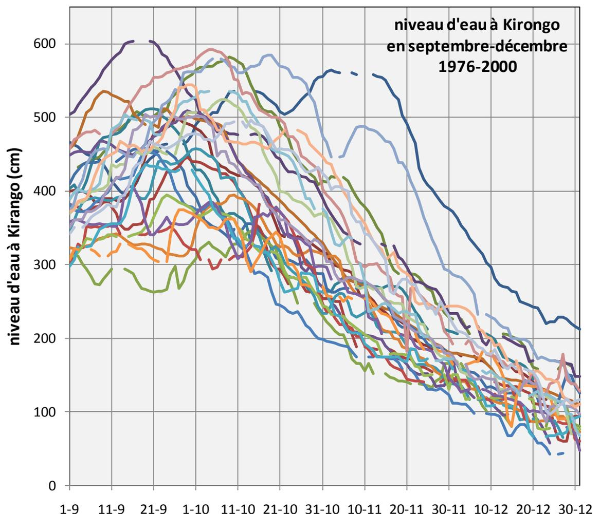
**Figure A5.** Water level at Kirango, just downstream of the Markala dam, such as measured between 1-1-1976 and 31-12-2000. The graph shows the daily measurements for the period 1 September – 31 December. Data from DNH.
